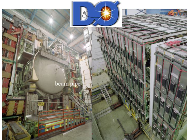
Figure 6: Pictures of DØ detector. The left picture shows the (relatively) small pipe that the colliding beams travel through.
